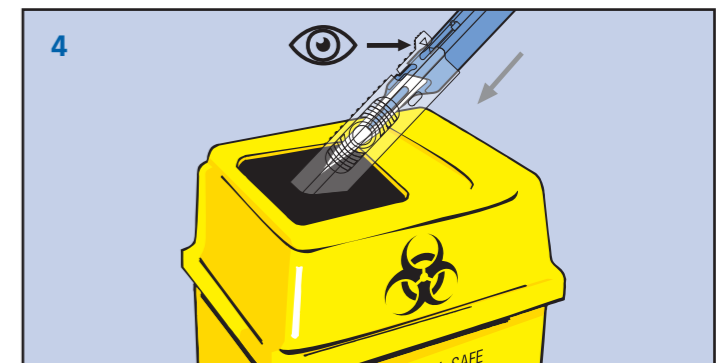
4 A visual check is recommended to ensure that the arrows on the handle and guard are aligned. This indicates that the final 'LOCK' position is activated, the guard cannot be retracted, and no further scalpel intervention is possible. The scalpel is then ready for disposal in an appropriate sharps' container when all counts have concluded.
